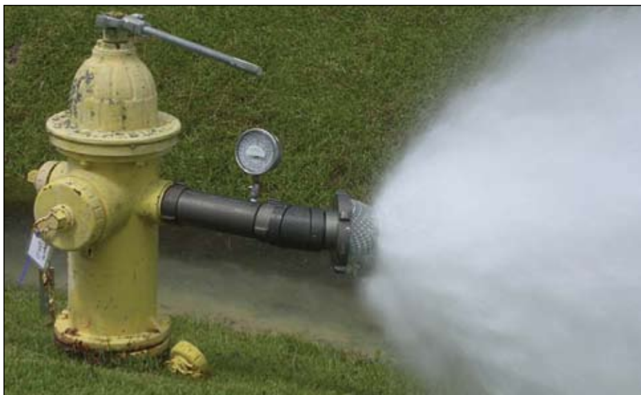
Figure 2. An integrated Pitot gauge and a wire-cage diffuser were installed on two flow hydrants.
