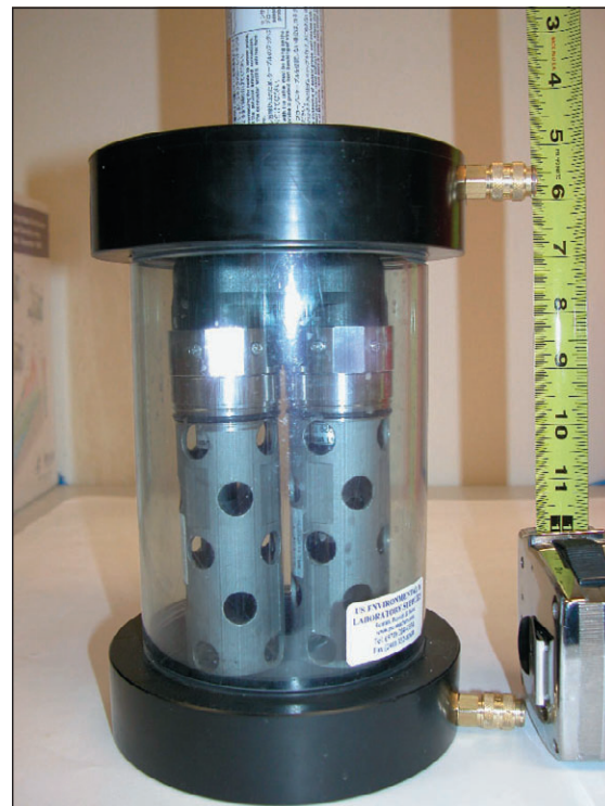
Figure 7-28. Horiba W-23XD Dual Probe Ion Detector Inside Flow Cell.
