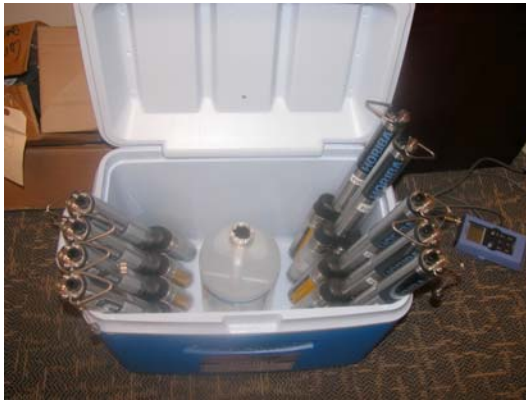
Figure 6. Photograph showing use of a water bath for calibrating multiple loggers.
